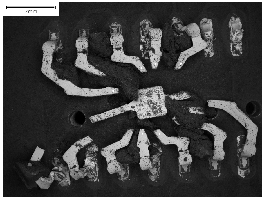
Figure 2. The interior of the controller integrated circuit
