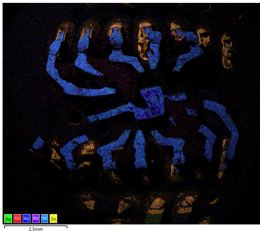
Figure 3. Distribution of elements on the surface of an integrated circuit
